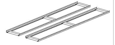
**5.** With the help of an associate, raise the two unit ends up and connect them with left to right channel beams (Ref. No. 3). Be sure the channel beams are fully seated.
