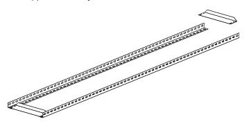
**3.** Place the remaining front-to-back support(s) evenly along the uprights. This forms one end of the tire rack.
