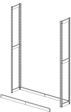
**6.** Attach the next section of left-to-right channel supports and place the shelf reinforcement in the middle the next shelf level.
